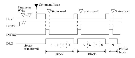
Figure 5.1 Execution example of READ MULTIPLE command
